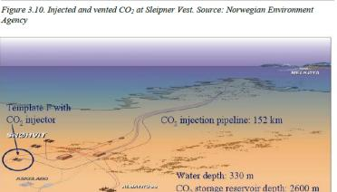
Figure 3.14. Snøhvit Field overview. Source: Statoil
