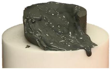
Left: Norwegian sensitive clay at the intact state,
