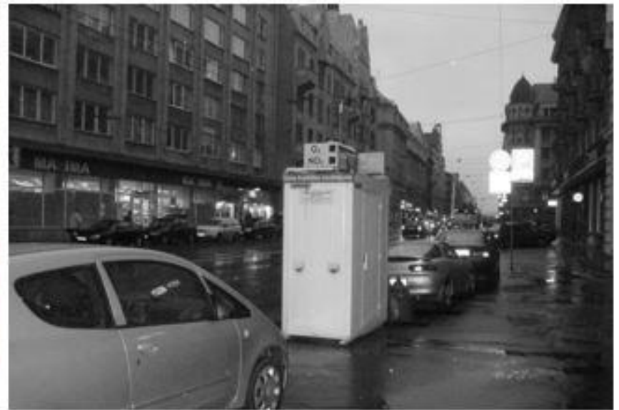
Street canyon AQMS on Brīvības Street 73 in city centre: open light beam DOAS technology, light beam 350 m
