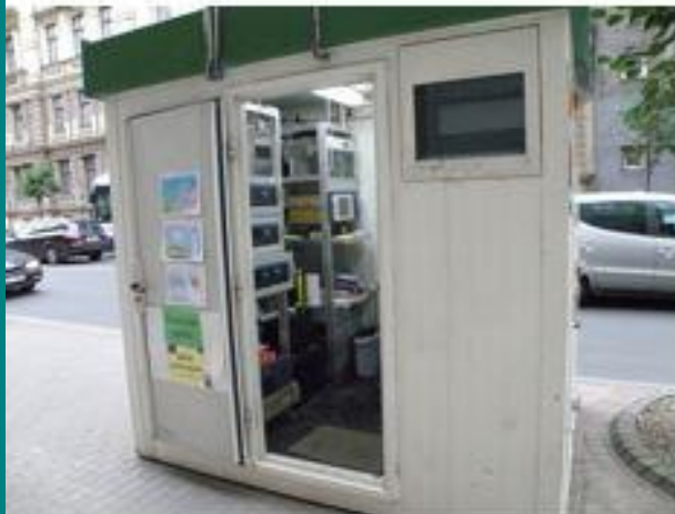
Street canyon on Kr.Valdemāra Street 18 in city centre: multi-instrumental classical point type AQMS
