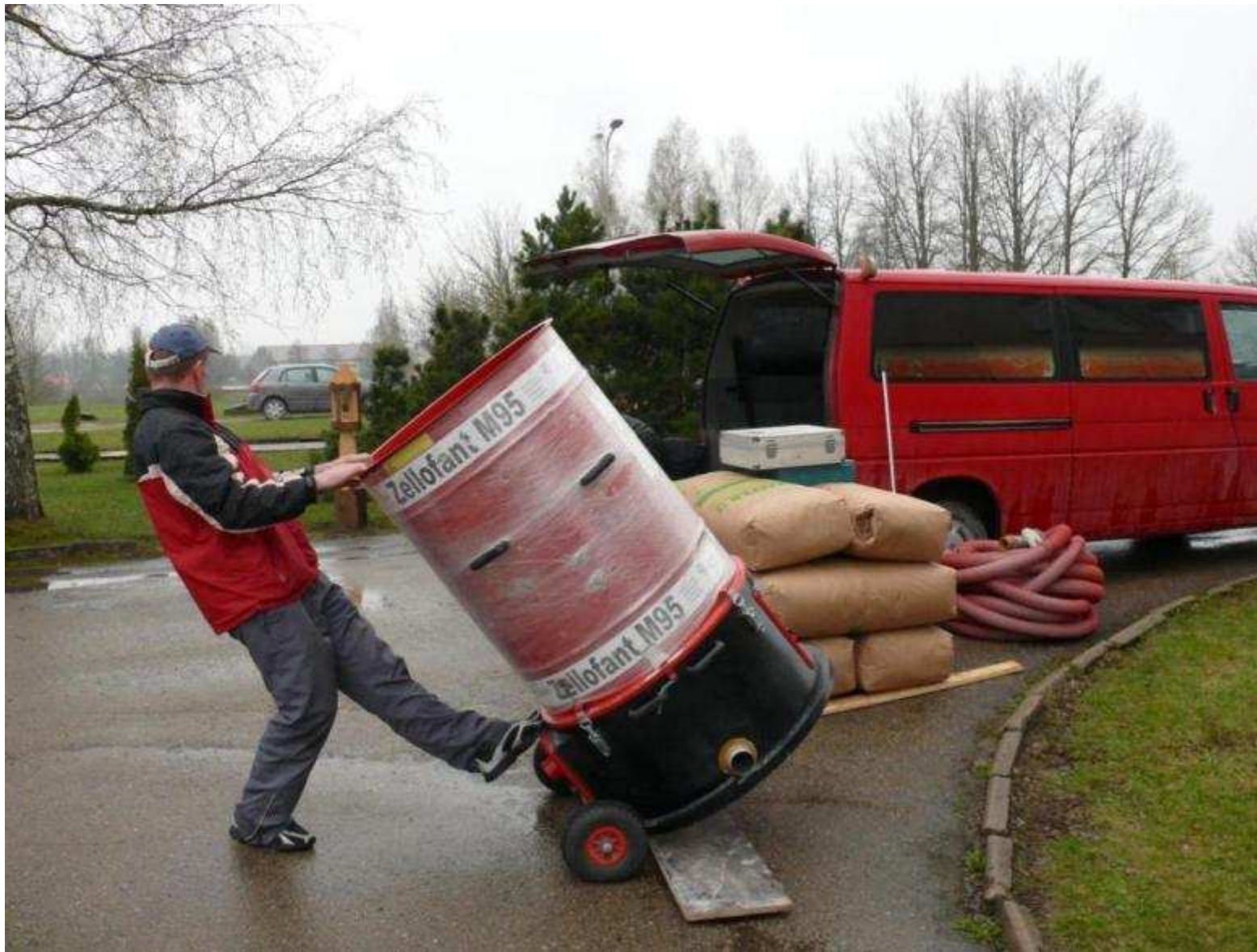
Cellulose blowing machine
